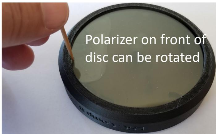
Rotating the front polarizer allows the developer to see how KaleidoFlow Rheoscopic Fluid shows different aspects of the flow conditions based on the orientation between the back and front polarizers.
